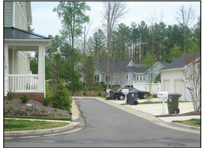
Rear-loaded garage serviced by an alley
